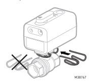
Fig. 4. Connect ball valve to actuator.
